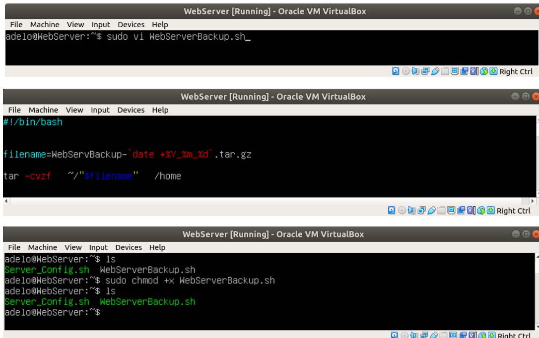
Figure 2.3: Creation of a Shell script that back up the entire contents of the home folder on WebServer
